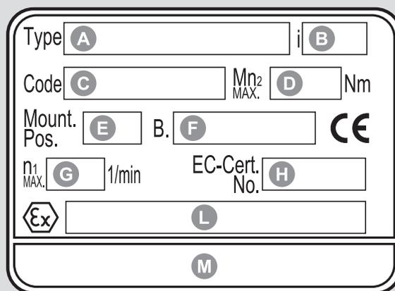
A diagram of a specific identification plate for speed reducers with the following fields:
